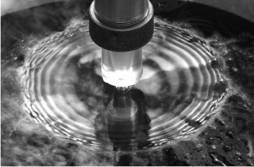
FIGURE 4. Vibrating liquid sheet as seen with the naked eye.
