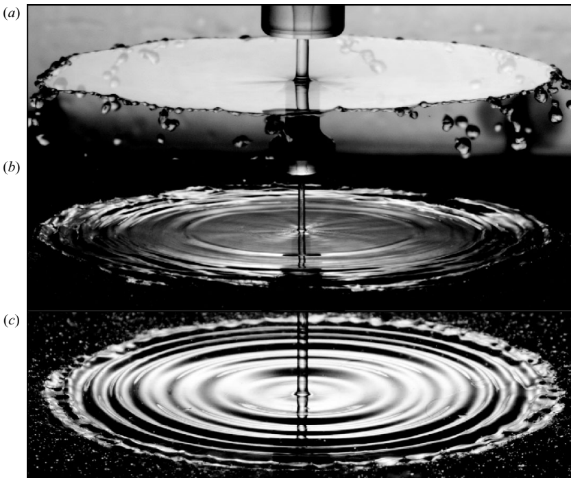
FIGURE 3. Axisymmetric liquid sheet states: (a) Smooth regime. (b) Flapping regime for larger Weber number (higher than 1000). (c) Perturbation of the smooth regime by vertically oscillating the impact cylinder.
